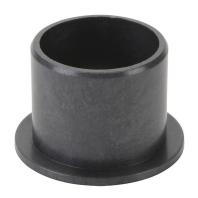
igus iglide series plain bearing, type G300 polymer, 3/4in inside diameter, 7/8in outside diameter, 3/4in overall length, flanged. Package of 5. For use with 3/4in diameter drylin R series shafts.
