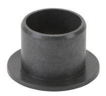
igus iglide series plain bearing, type G300 polymer, 1/2in inside diameter, 9/16in outside diameter, 1/2in overall length, flanged. Package of 10. For use with 1/2in diameter drylin R series shafts.
