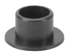
igus iglide series plain bearing, type G300 polymer, 1/4in inside diameter, 5/16in outside diameter, 1/4in overall length, flanged. Package of 10. For use with 1/4in diameter drylin R series shafts.
