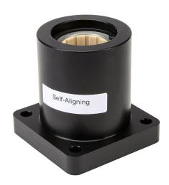
igus drylin R series plain bearing, type J polymer bearing, 1in inside diameter, 2-13/16in overall length, self-aligning housing, 4-bolt flange pillow block, anodized aluminum, flanged.
