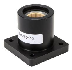
igus drylin R series plain bearing, type J polymer bearing, 3/4in inside diameter, 2-1/16in overall length, self-aligning housing, 4-bolt flange pillow block, anodized aluminum, flanged.
