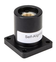
igus drylin R series plain bearing, type J polymer bearing, 1/2in inside diameter, 1-11/16in overall length, self-aligning housing, 4-bolt flange pillow block, anodized aluminum, flanged.
