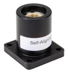
igus drylin R series plain bearing, type J polymer bearing, 1/2in inside diameter, 1-11/16in overall length, self-aligning housing, 4-bolt flange pillow block, anodized aluminum, flanged.
