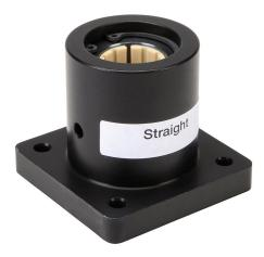
igus drylin R series plain bearing, type J polymer bearing, 3/4in inside diameter, 2-1/16in overall length, fixed housing, 4-bolt flange pillow block, anodized aluminum, flanged.
