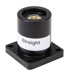
igus drylin R series plain bearing, type J polymer bearing, 1/2in inside diameter, 1-11/16in overall length, fixed housing, 4-bolt flange pillow block, anodized aluminum, flanged.
