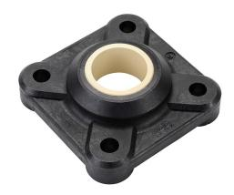
igus igubal E series mounted spherical bearing, type L280 polymer bearing, 1in inside diameter, 4-bolt flange, igumid G polymer.
