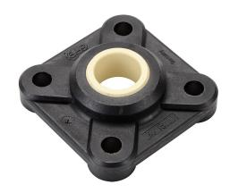
igus igubal E series mounted spherical bearing, type L280 polymer bearing, 3/4in inside diameter, 4-bolt flange, igumid G polymer.
