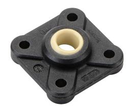
igus igubal E series mounted spherical bearing, type L280 polymer bearing, 1/4in inside diameter, 4-bolt flange, igumid G polymer. Package of 4.
