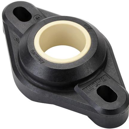
igus igubal E series mounted spherical bearing, type L280 polymer bearing, 1in inside diameter, 2-bolt flange, igumid G polymer.
