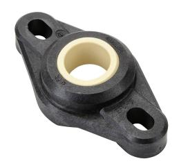
igus igubal E series mounted spherical bearing, type L280 polymer bearing, 3/4in inside diameter, 2-bolt flange, igumid G polymer.
