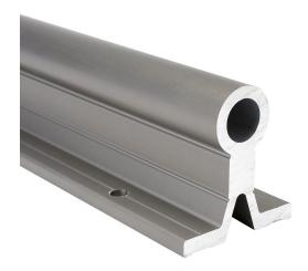
igus drylin R series supported shaft, 6060/6061 aluminum, 450-550 HV, hard-anodized aluminum, 1in diameter, 250mm length. For use with 1in drylin R series bearings.
