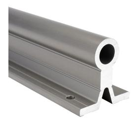
igus drylin R series supported shaft, 6060/6061 aluminum, 450-550 HV, hard-anodized aluminum, 1in diameter, 1000mm length. For use with 1in drylin R series bearings.
