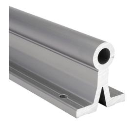
igus drylin R series supported shaft, 6060/6061 aluminum, 450-550 HV, hard-anodized aluminum, 3/4in diameter, 500mm length. For use with 3/4in drylin R series bearings.
