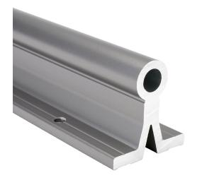
igus drylin R series supported shaft, 6060/6061 aluminum, 450-550 HV, hard-anodized aluminum, 3/4in diameter, 250mm length. For use with 3/4in drylin R series bearings.
