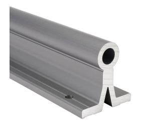
igus drylin R series supported shaft, 6060/6061 aluminum, 450-550 HV, hard-anodized aluminum, 3/4in diameter, 1000mm length. For use with 3/4in drylin R series bearings.
