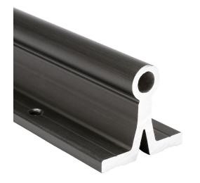
igus drylin R series supported shaft, 6060/6061 aluminum, 450-550 HV, hard-anodized aluminum, 1/2in diameter, 500mm length. For use with 1/2in drylin R series bearings.
