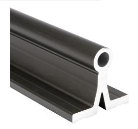
igus drylin R series supported shaft, 6060/6061 aluminum, 450-550 HV, hard-anodized aluminum, 1/2in diameter, 250mm length. For use with 1/2in drylin R series bearings.
