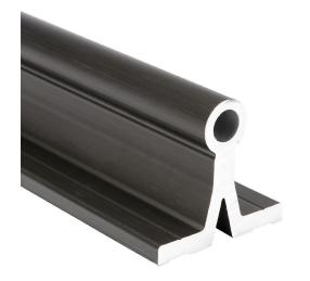
igus drylin R series supported shaft, 6060/6061 aluminum, 450-550 HV, hard-anodized aluminum, 1/2in diameter, 250mm length. For use with 1/2in drylin R series bearings.
