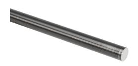
igus drylin R series round connecting shaft, 6060/6061 aluminum, 450-550 HV, hard-anodized aluminum, 10mm diameter, 500mm length. For use with all ZLW series actuators.
