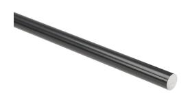
igus drylin R series round connecting shaft, 6060/6061 aluminum, 450-550 HV, hard-anodized aluminum, 10mm diameter, 1000mm length. For use with all ZLW series actuators.
