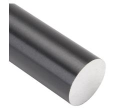
igus drylin R series round shaft, 6060/6061 aluminum, 450-550 HV, hard-anodized aluminum, 1in diameter, 500mm length. For use with 1in drylin R series, igus igubal E and K series and iglide bearings.
