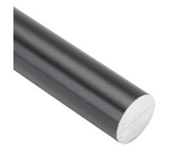
igus drylin R series round shaft, 6060/6061 aluminum, 450-550 HV, hard-anodized aluminum, 3/4in diameter, 250mm length. For use with 3/4in drylin R series, igus igubal E and K series and iglide bearings.
