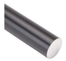
igus drylin R series round shaft, 6060/6061 aluminum, 450-550 HV, hard-anodized aluminum, 3/4in diameter, 1000mm length. For use with 3/4in drylin R series, igus igubal E and K series and iglide bearings.
