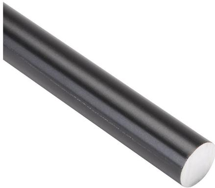
igus drylin R series round shaft, 6060/6061 aluminum, 450-550 HV, hard-anodized aluminum, 1/2in diameter, 500mm length. For use with 1/2in drylin R series, igus igubal E and K series and iglide bearings.
