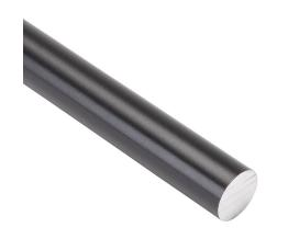
igus drylin R series round shaft, 6060/6061 aluminum, 450-550 HV, hard-anodized aluminum, 1/2in diameter, 1000mm length. For use with 1/2in drylin R series, igus igubal E and K series and iglide bearings.
