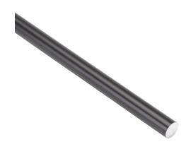
igus drylin R series round shaft, 6060/6061 aluminum, 450-550 HV, hard-anodized aluminum, 1/4in diameter, 500mm length. For use with 1/4in drylin R series, igus igubal E and K series and iglide bearings.
