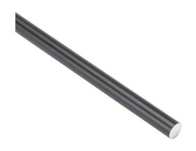
igus drylin R series round shaft, 6060/6061 aluminum, 450-550 HV, hard-anodized aluminum, 1/4in diameter, 250mm length. For use with 1/4in drylin R series, igus igubal E and K series and iglide bearings.
