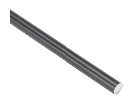
igus drylin R series round shaft, 6060/6061 aluminum, 450-550 HV, hard-anodized aluminum, 1/4in diameter, 1000mm length. For use with 1/4in drylin R series, igus igubal E and K series and iglide bearings.
