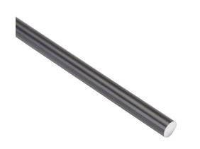
igus drylin R series round shaft, 6060/6061 aluminum, 450-550 HV, hard-anodized aluminum, 1/4in diameter, 1000mm length. For use with 1/4in drylin R series, igus igubal E and K series and iglide bearings.
