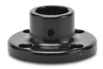
WERMA mounting base, tube mount, 25mm diameter, black, aluminum. For use with 50mm or 70mm terminal elements. Rubber seal included.
