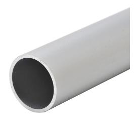
WERMA extension tube, 25mm diameter, 400mm length, silver, aluminum. For use with 50mm or 70mm terminal elements.
