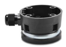
WERMA magnetic contact box, black, polyamide. For use with 50mm and 70mm terminal elements. Mounting hardware, seal and M16  $\times$  1.5mm cable gland included.
