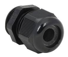
WERMA cable gland, M25 x 1.5mm thread type, polyamide, black, accepts 8 to 17mm diameter cable, IP68.
