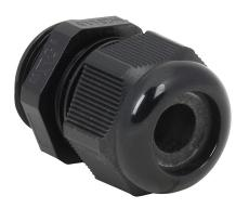
WERMA cable gland, M25 x 1.5mm thread type, polyamide, black, accepts 8 to 17mm diameter cable, IP68.
