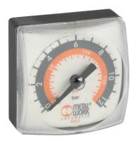
Metal Work pneumatic mechanical pressure gauge, 40mm x 40mm, 0 to 180 psi, G1/8 male BSPP process connection, center back mount.
