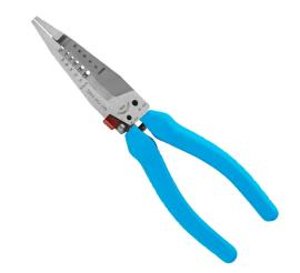
CHANNELLOCK multi-purpose wiring tool, compatible with data & communications cable and round wire, comfort grip, curved shear cutting edges, 20-12 AWG stranded and 18-10 AWG solid wire stripping capacity, 10 AWG cutting capacity.
