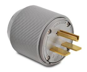
Bryant industrial heavy duty straight blade plug, 30A, 250 VAC, 1-phase, 2-pole, 3-wire, NEMA 6-30, accepts cord size 0.42-1.32in, thermoplastic housing, gray.
