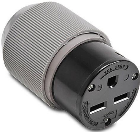
Bryant industrial heavy duty straight blade connector, 30A, 250 VAC, 1-phase, 2-pole, 3-wire, NEMA 6-30, accepts cord size 0.42-1.32in, thermoplastic housing, gray.
