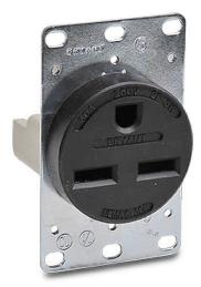
Bryant industrial heavy duty single straight blade receptacle, 30A, 250 VAC, 1-phase, 2-pole, 3-wire, NEMA 6-30, thermoplastic molded housing, gray.
