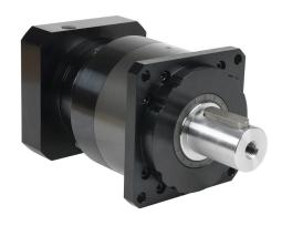
LS Electric high-precision planetary gearbox, 15:1 ratio, inline, 55mm diameter output shaft, nominal output torque 897 N-m (7939 lb-in), 2-stage, 180mm frame. For use with APM-FF series 7.5 kW motors.
