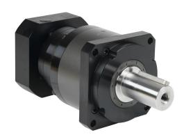
LS Electric high-precision planetary gearbox, 20:1 ratio, inline, 40mm diameter output shaft, nominal output torque 295 N-m (2611 lb-in), 2-stage, 142mm frame. For use with APM-FE series 1.6 kW motors.
