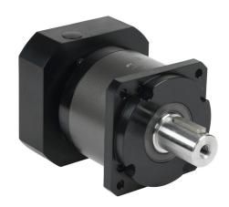
LS Electric high-precision planetary gearbox, 10:1 ratio, inline, 32mm diameter output shaft, nominal output torque 262 N-m (2319 lb-in), 1-stage, 115mm frame. For use with APM-FE series 1.6 kW motors.
