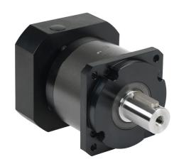
LS Electric high-precision planetary gearbox, 5:1 ratio, inline, 32mm diameter output shaft, nominal output torque 332 N-m (2939 lb-in), 1-stage, 115mm frame. For use with APM-FE series 1.6 kW motors.
