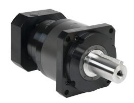
LS Electric high-precision planetary gearbox, 20:1 ratio, inline, 40mm diameter output shaft, nominal output torque 295 N-m (2611 lb-in), 2-stage, 142mm frame. For use with APM-FE series 2.2 kW motors.
