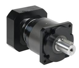
LS Electric high-precision planetary gearbox, 20:1 ratio, inline, 32mm diameter output shaft, nominal output torque 295 N-m (2611 lb-in), 2-stage, 115mm frame. For use with APM-FE series 900W and 1.5 kW motors.
