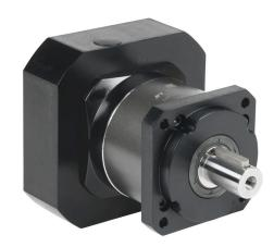
LS Electric high-precision planetary gearbox, 10:1 ratio, inline, 22mm diameter output shaft, nominal output torque 121 N-m (1071 lb-in), 1-stage, 90mm frame. For use with APM-FE series 900W and 1.5 kW motors.
