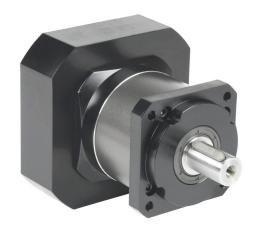
LS Electric high-precision planetary gearbox, 5:1 ratio, inline, 22mm diameter output shaft, nominal output torque 160 N-m (1416 lb-in), 1-stage, 90mm frame. For use with APM-FE series 900W and 1.5 kW motors.
