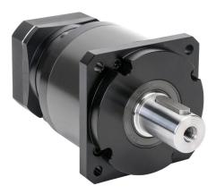
LS Electric high-precision planetary gearbox, 20:1 ratio, inline, 32mm diameter output shaft, nominal output torque 295 N-m (2611 lb-in), 2-stage, 115mm frame. For use with FCL series 750W and 1 kW motors.
