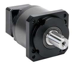
LS Electric high-precision planetary gearbox, 20:1 ratio, inline, 22mm diameter output shaft, nominal output torque 143 N-m (1266 lb-in), 2-stage, 90mm frame. For use with FBL series 100W-400W motors.
