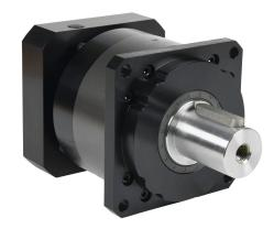
LS Electric high-precision planetary gearbox, 10:1 ratio, inline, 55mm diameter output shaft, nominal output torque 980 N-m (8674 lb-in), 1-stage, 180mm frame. For use with APM-FF series 7.5 kW motors.
